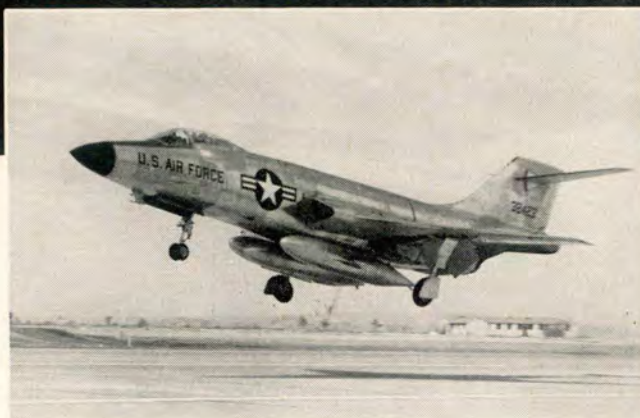
The F-101, new USAF long-range, supersonic penetration fighter, has gained increased range by the addition of three external fuel tanks.
