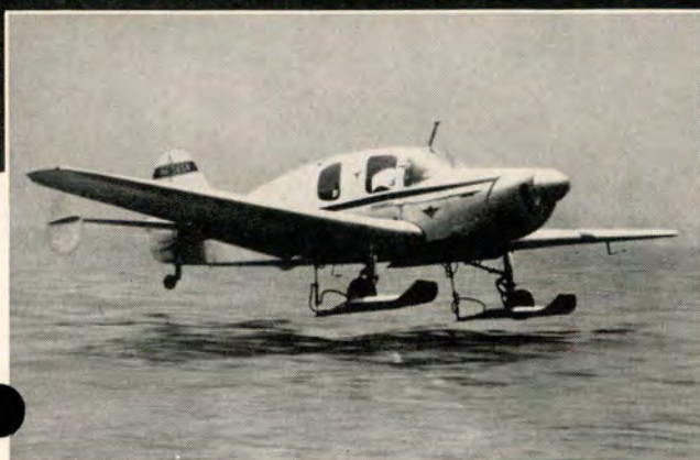
A Bellanca, equipped with a retractable hydro-lift gear, lands on the water. By maintaining 15 mph, a pilot can taxi the plane onto beach.
